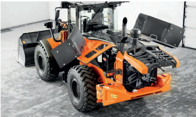
Engine cover enables convenient access for daily inspections.
