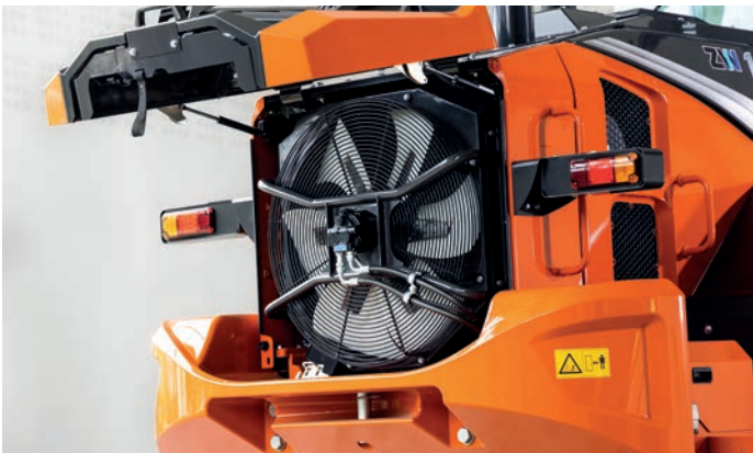
Intelligent fan operation system prevents radiators clogging.
