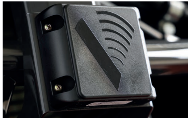
Rear obstacle detection system enhances safety on the job site.
